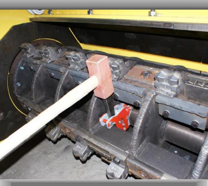
Old tools can be easily removed with a press, quick and easy insertion of new tools.
