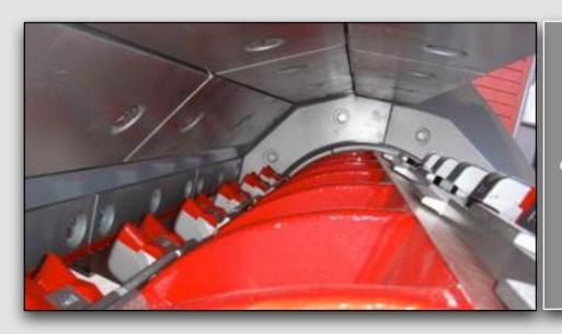
Even the armour plates of the crushing chamber are very easy to replace
