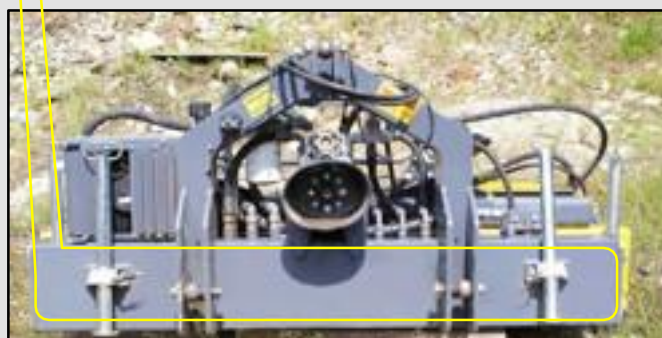
Oil tank with a capacity of 95 litres
