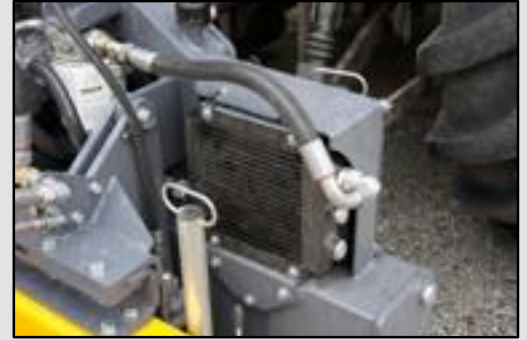
Independent oil cooler with fan and sheet metal cladding
