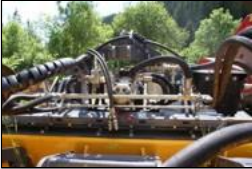
3 hydraulic pumps – driven via the universal joint shaft
